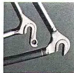
Stainless steel dropouts prevent tip damage during rapid wheel changes.
