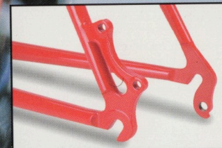
International Standard disc brake dropouts on the Ala Carte Mountain frame.
