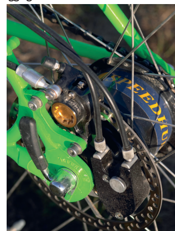
Below left: Single chainring means no chain line issues. Below right: Rohloff's Speedhub is a major investment but looks to pay long-term dividends by its immunity to cassette and derailleur-clogging mud
