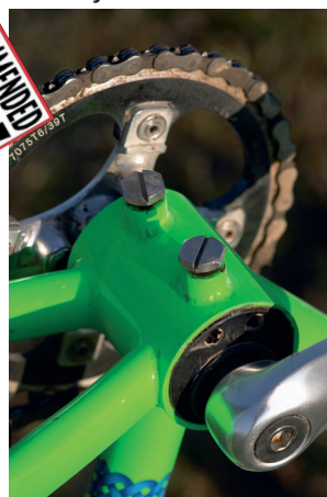
Below left: Single chainring means no chain line issues. Below right: Rohloff's Speedhub is a major investment but looks to pay long-term dividends by its immunity to cassette and derailleur-clogging mud
