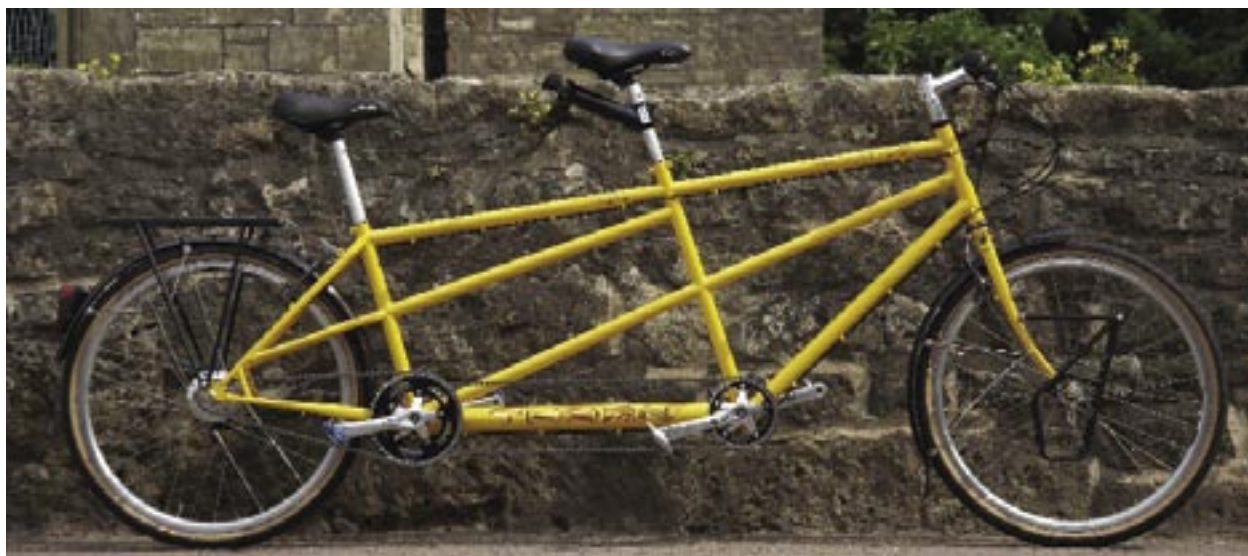
(Top) The Dawes' adjustable stem allows position tweaks but is better swapped for a rigid one long-term (Above) The budget sprung seatpost works okay
