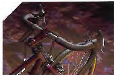
SR Fat Drop bars with Modolo bend, Flip Flop stem, and SunTour Command shifters make this bike a navigational dream.
