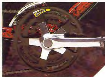
SR XCU Crankset with alloy crankarms and round "Powering" chainrings afford smooth pedaling and positive shifting.
