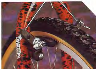
Low Profile DiaCompe XCU front cantilever is narrow, easily adjustable and provides excellent braking power.
