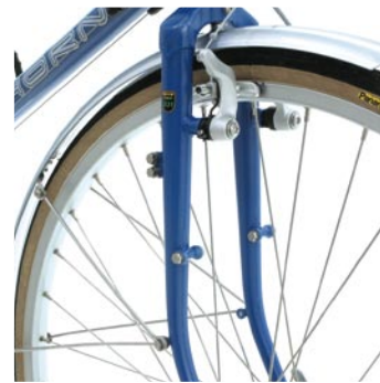
Lo loader and bottle generator dynamo bosses.
