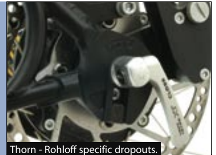
Thorn - Rohloff specific dropouts.
