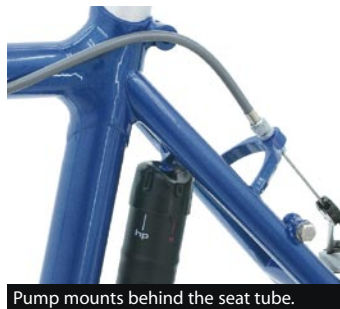
Pump mounts behind the seat tube.
