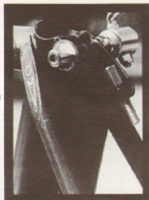
The exclusive Mountaineer seat binder locks the release lever position, hangs the rear brake cable and holds a pump all at once.
